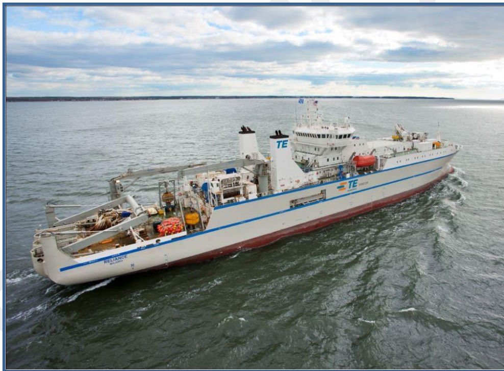
The cable laying vessel RESPONDER with its length of 145 m transporting equipment and personnel for the reconstruction of the hydroacoustic listening station.
